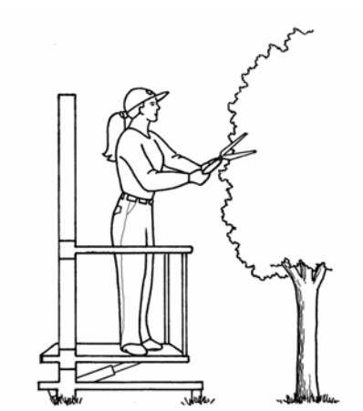
Figure 6 - Adjustable platform reduces stooping and reaching
