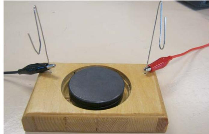
Adjust current and voltage knobs so that  $\sim 12V$  is applied to the motor. You will likely need to adjust the voltage, once you test your motor.
