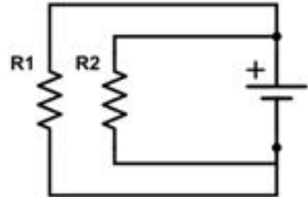
**With power supply OFF**, use both resistors and the power supply to connect the circuit as shown above.
