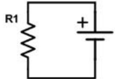
Connect the “+” on the power supply to **one** of the terminals of the resistor box, and connect the other terminal of that resistor back to the “-” **of the supply**. This completes a simple electrical circuit.
