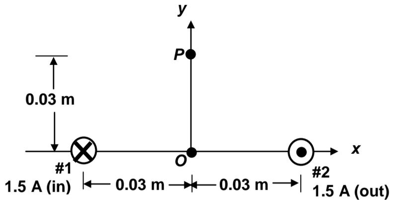
(a) On the diagram, draw and label the contributions from wire #1 and wire #2 to the magnetic field at point  $P$  which is located at  $x = 0$  cm,  $y = 0.03$  m as shown.
