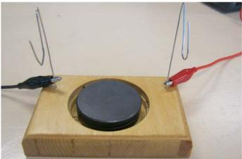
Adjust current and voltage knobs so that  $\sim 12V$  is applied to the motor. You will likely need to adjust the voltage, once you test your motor.
