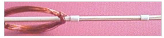
The thin copper wire provided has a very thin enamel coating that prevents it from short circuiting (current unintentionally flowing between coils). Part of producing enough torque to rotate the coil as desired means there needs to be a number of coils.
