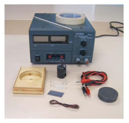
To build the motor successfully, the coil must be balanced and attached to the wooden stick so they can rotate smoothly on the wire stands. There are many elements required to build the motor and for it to operate successfully.
