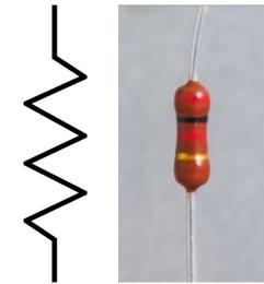
Resistors vary in design based on how much electrical resistance they provide, and the power they may be subjected to in the circuit.
