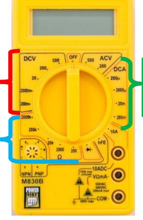
Measures DC current from 200 microamps  $(\mu A)$  to 200 milliamps (mA).
