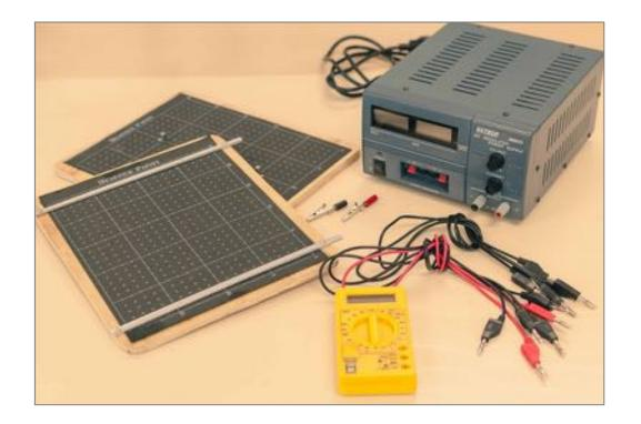
Your conductive paper has one of the following patterns. The metal components attached are referred to as **electrodes**. We'll connect our power supply leads to these electrodes to supply voltage.
