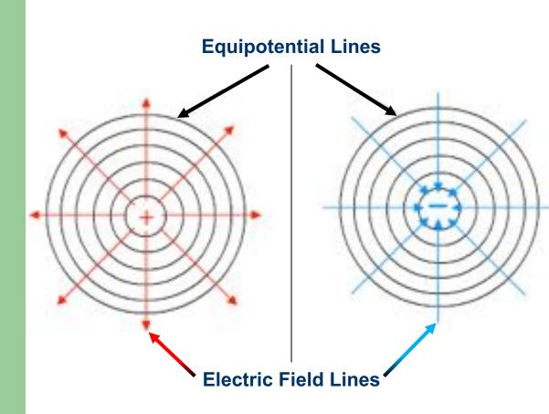
Equipotential lines (black) and electric field lines (coloured) for positive and negative point charges are described as shown.
