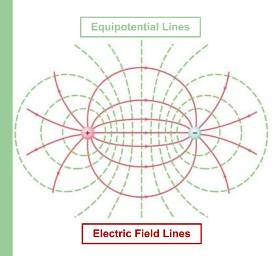
Equipotential lines are always perpendicular to electric field lines, even in more complicated scenarios.
