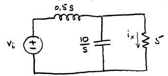
4) In the circuit shown,  $\omega = 5000$  rad/s. Using phasors find the phasor voltage  $V_I$  and the voltage  $V_I(t)$ .
