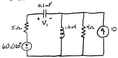
5) At t = 0 the switch is suddenly closed. There is no energy stored in the circuit for t < 0. Using the technique of your choice, find  $i_L$  for t > 0.
