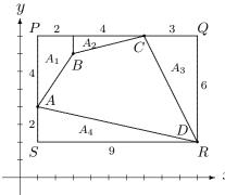
Construct the rectangle PQRS as shown and draw a perpendicular from B to PQ. Then the area of the quadrilateral ABCD is equal to area of the rectangle less the areas of the trapezoid and triangles with areas  $A_1$ ,  $A_2$ ,  $A_3$  and  $A_4$  as indicated,
