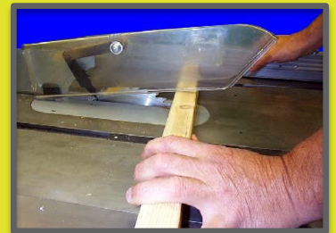
Self-adjusting guard for table saw blade
