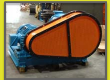
Guard enclosing a power transmission apparatus
