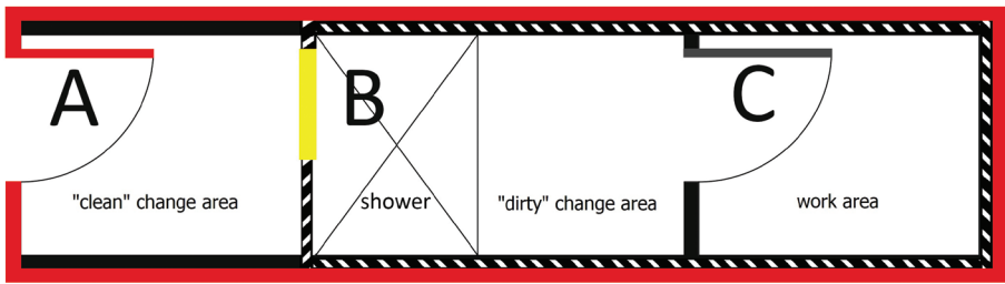
Figure 3–8: Representative Diagram of Anteroom Spaces in a Containment Level 3 (CL3) Zone Identifying the Critical Door.
