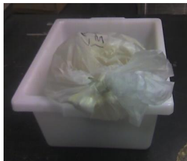
Figure 3: Use of secondary containment
