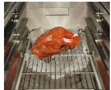
Figure 4: No secondary containment
