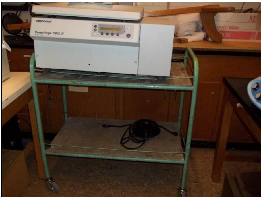
Photograph 39: Room SN3119A. Asbestos containing transite cart, in poor condition
