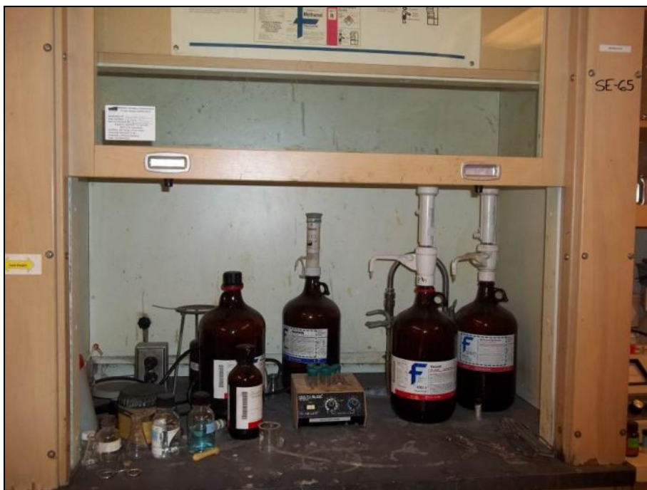
Photograph 9: Room SN1049. Asbestos containing transite fume hood. Sample SN-69.
