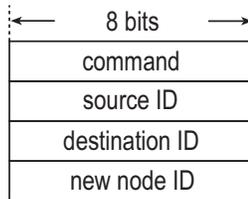
Fig. 3. Packet format of incorporating new detection node
