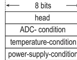
Fig. 5. Packet format of condition information
