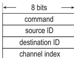
Fig. 6. Packet format of channel changing and release
