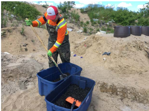
Picture 2. Photograph showing mixing of biochar with sand
