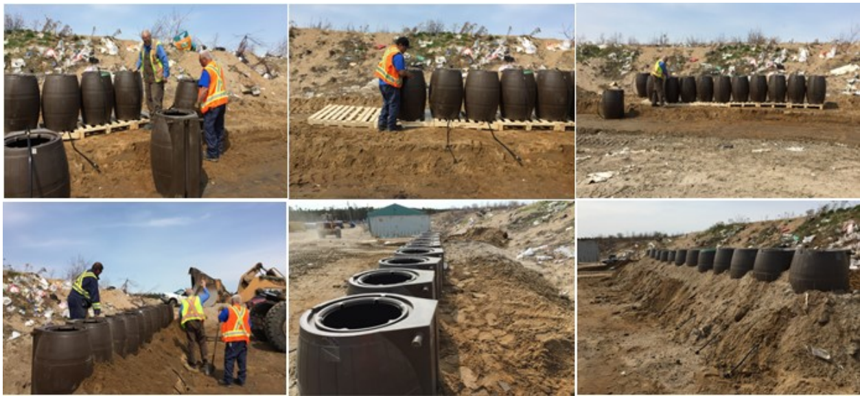
Picture 1. Photographs showing preparation of berm and setting up rain barrels for experimentation
