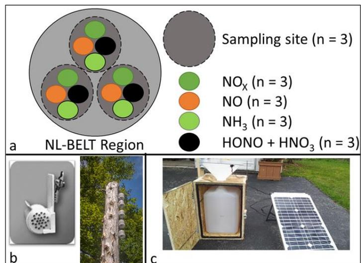
**Figure 2.** Installed in each NL-BELT region with statistical replication within and between sampling sites (a) are Ogawa<sup>®</sup> passive diffusion samplers for reactive gases (b) and custom-built automated precipitation collectors, (c) for through-fall (n = 3) and open fall (n = 3) rain samples.
