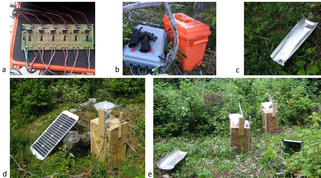
**Figure 4.** Automated precipitation samplers. In-house electronics design (a) were deployed in environmentally protected cases (b) to interface with the precipitation sensor (c) and solar panel (d) such that precipitation events (e) could be captured over a period of up to a month.
