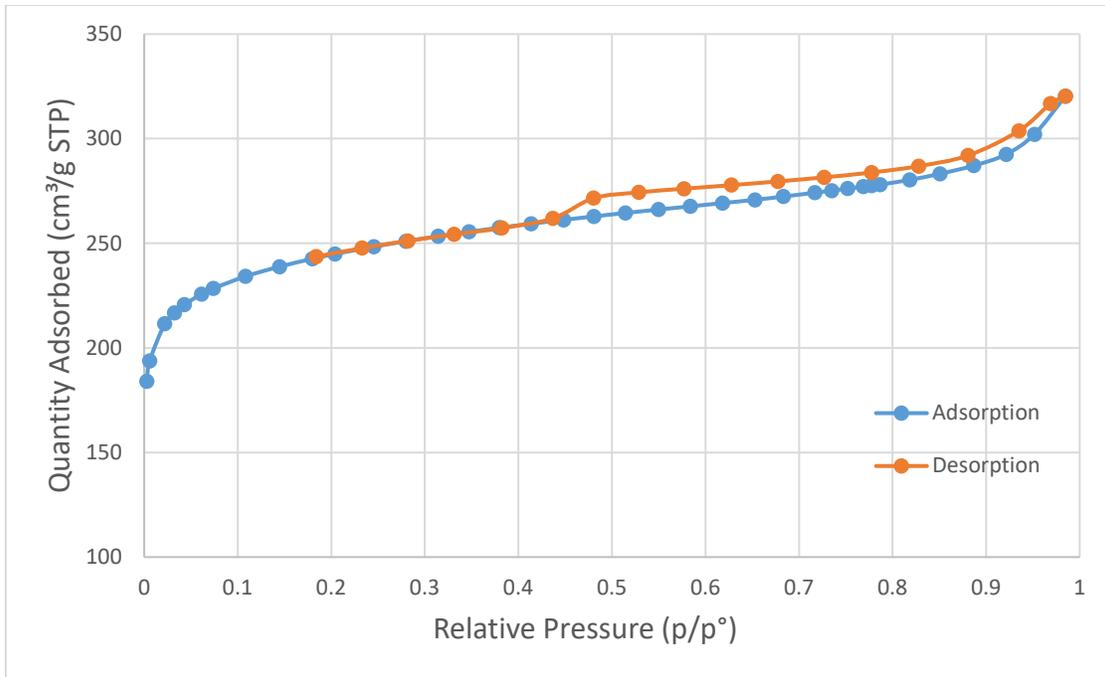
Figure 2-10: N<sub>2</sub> adsorption-desorption isotherm linear plot of CSA (Zhang et al., 2017)
