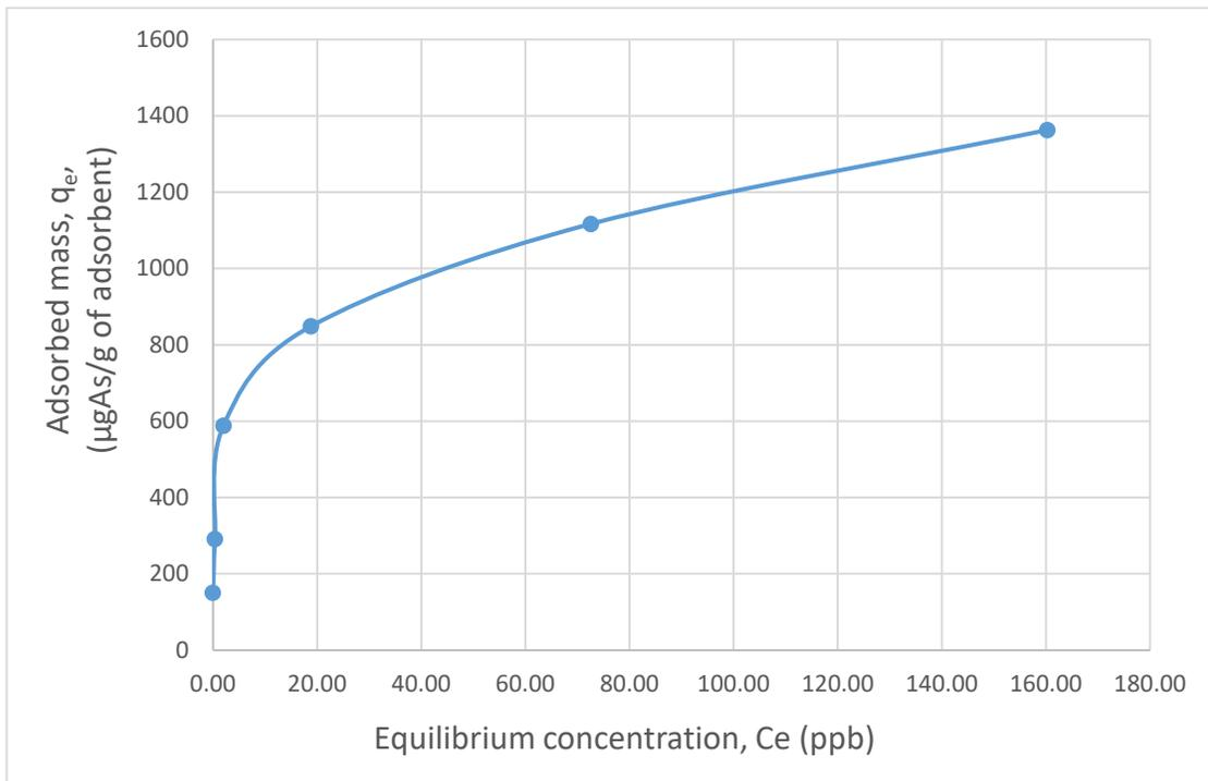
Figure 3-2: Isotherm curve of arsenic removal from synthesized water ( $\text{Na}_2\text{HAsO}_4 \cdot 7\text{H}_2\text{O}$ , 1 ppm)
