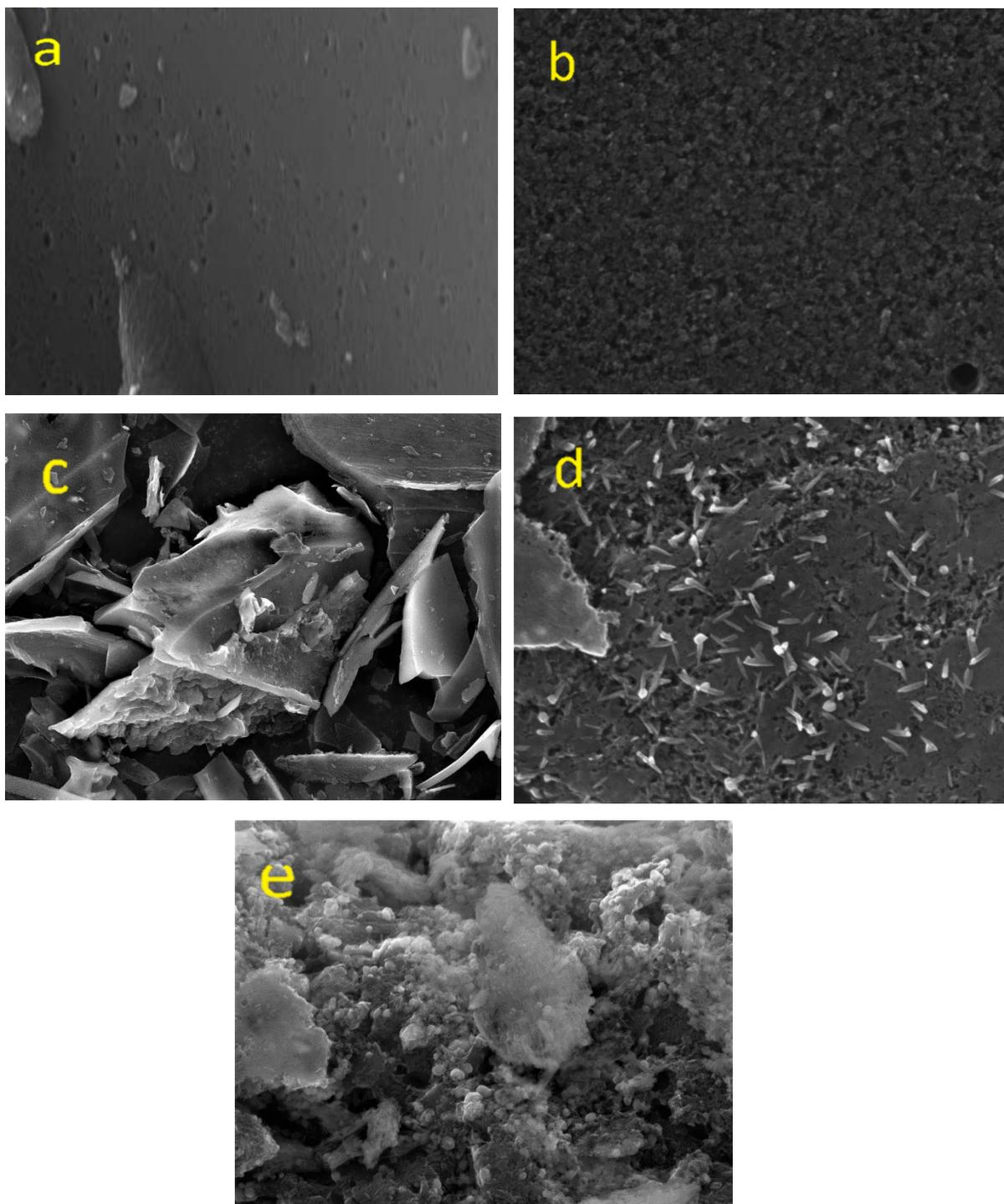
Figure 2-8: SEM image of carbon samples: a) CBPP fly ash before activation, b) CSAC after activation at 850°C, c) CSAC impregnated with 0.01M  $\text{FeCl}_3$ , d) CSAC impregnated with 0.1M  $\text{FeCl}_3$ , e) CSAC impregnated with 1M  $\text{FeCl}_3$
