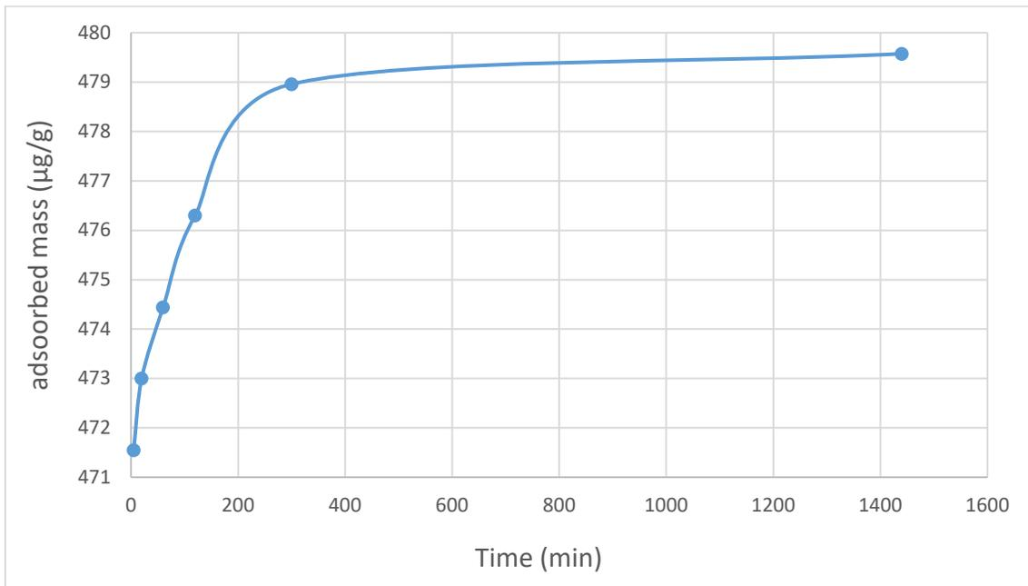
Figure 3-4: Sorption kinetic of synthesized arsenic contaminated water ( $\text{Na}_2\text{HAsO}_4 \cdot 7\text{H}_2\text{O}$ , 1 ppm)
