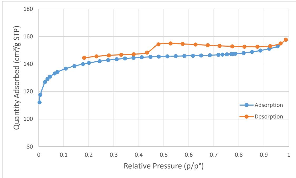
Figure 2-9: N<sub>2</sub> adsorption-desorption isotherm linear plot of raw and cleaned CBPP fly ash (Zhang et al., 2017)
