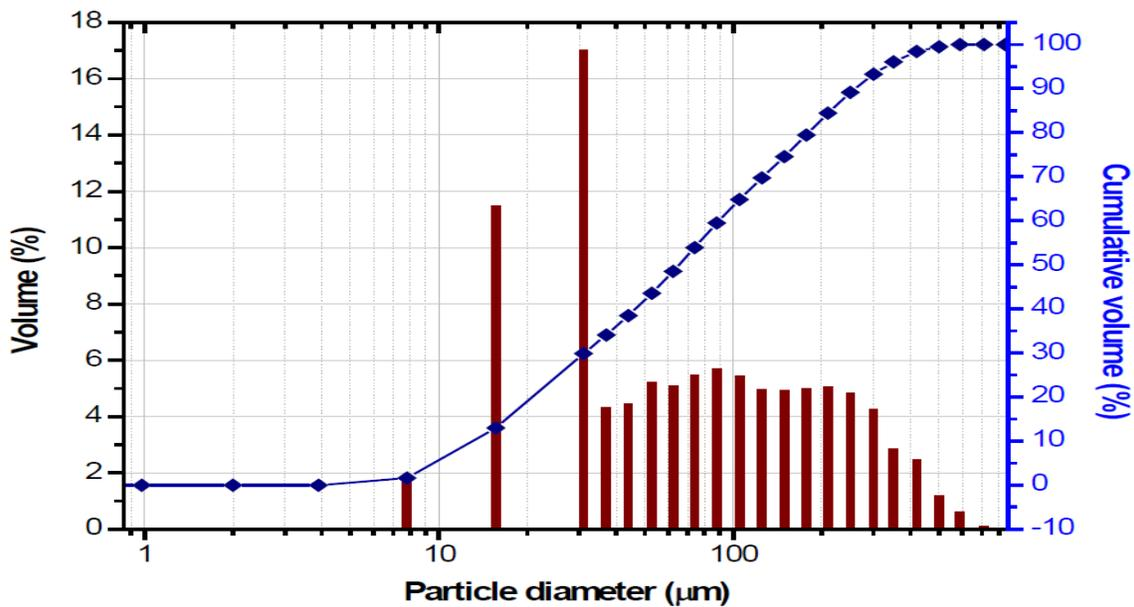
Figure 2-1: particle size distribution of CBPP fly ash after grinding (Zhang *et al.*, 2017)
