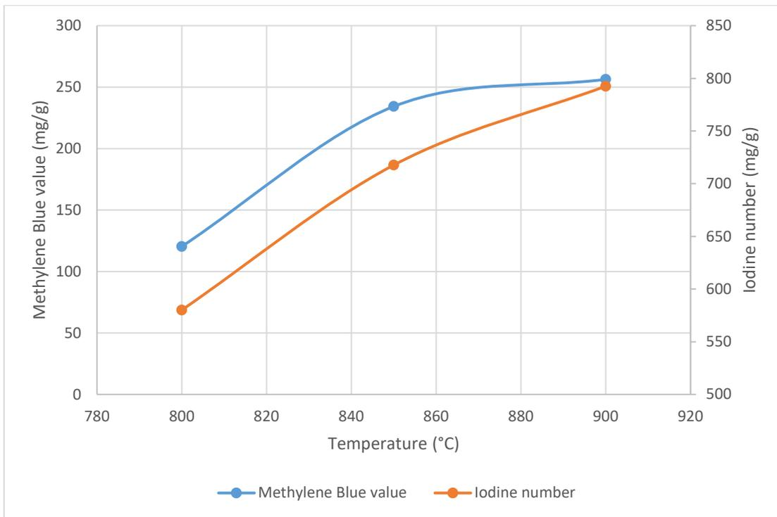
Figure 2-3: MBV and IN of CSAC at different temperatures (constant time)
