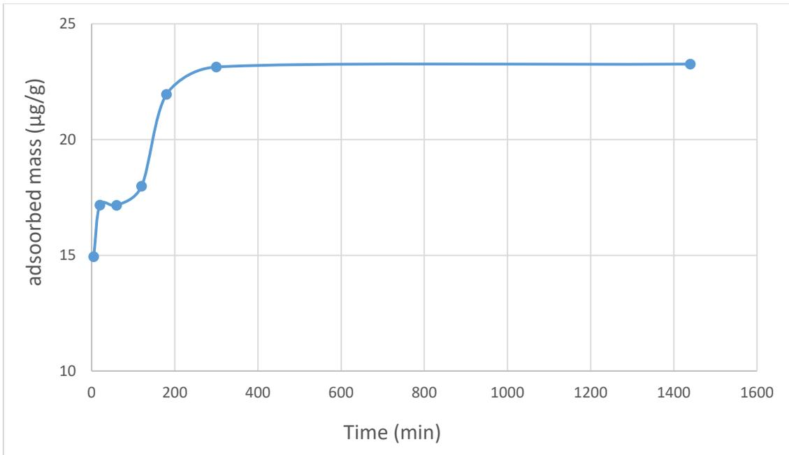
Figure 3-3: Sorption kinetic of local well water
