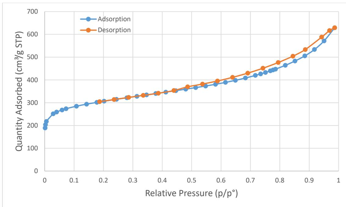
Figure 2-12: N<sub>2</sub> adsorption-desorption isotherm linear plot of CSAC impregnated with 0.1 M FeCl<sub>3</sub>
