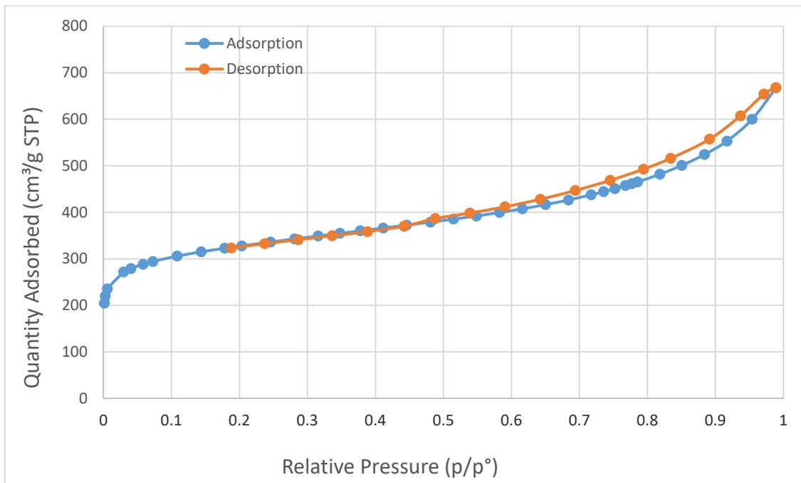
Figure 2-11: N<sub>2</sub> adsorption-desorption isotherm linear plot of CSAC
