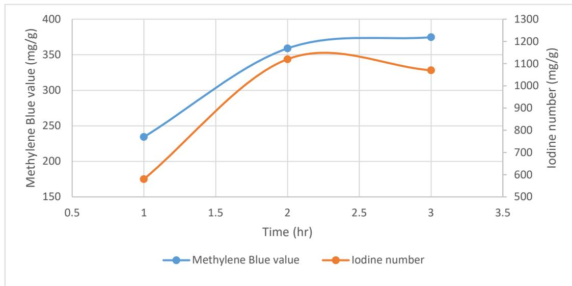
Figure 2-5: MBV and IN changes with time for CSAC at 850°C
