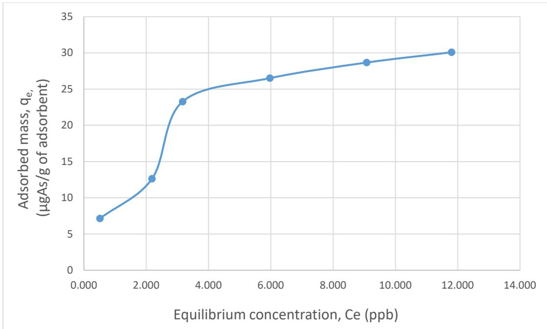
Figure 3-1: Isotherm curve of arsenic removal from local well water
