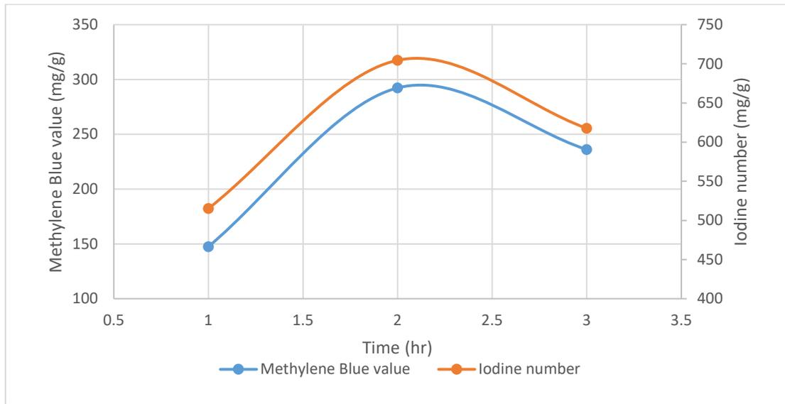
Figure 2-4: MBV and IN changes with time for CAC at 850°C (Zhang et al., 2017)
