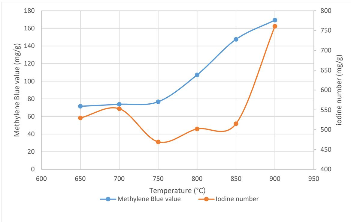
Figure 2-2: MBV and IN of CSA at different temperatures (constant time)(Zhang et al., 2017)
