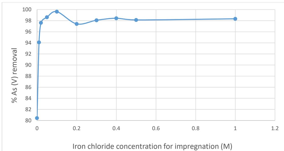
Figure 2-6: Percentage of arsenic (V) removal using CSAC samples impregnated with different iron chloride concentration
