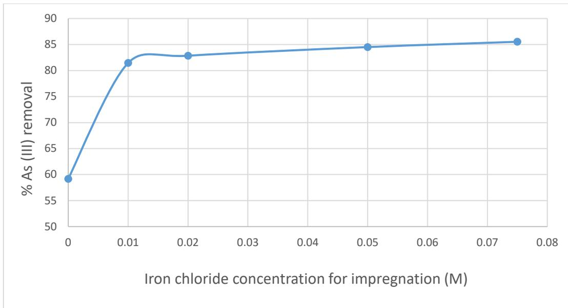
Figure 2-7: Percentage of arsenic (III) removal using CSAC samples impregnated with different iron chloride concentration
