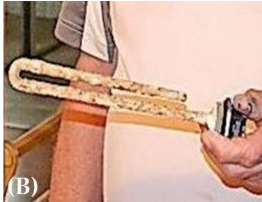
(A) Difference between new filters (white) for a reverse osmosis water filtration system and the old filters covered with a brownish “slimy” substance). (B) Corroded part of a two-year-old water heater - Courtesy Derek Montague.
