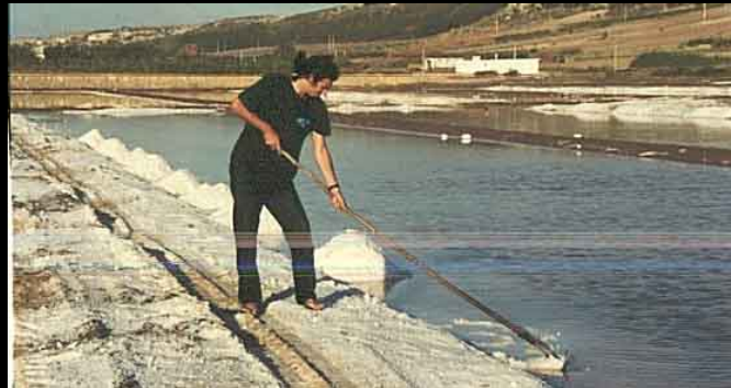
Figure 12: Open pan evaporation for production of salt.
