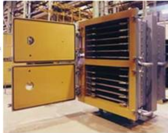
Figure 3: Schematic and photograph of a tray dryer.
