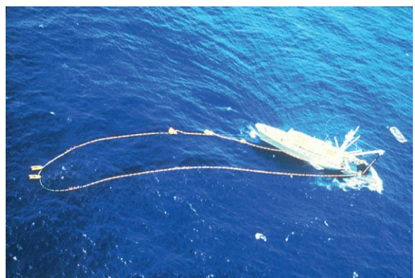
Figure 2 Backdown procedure in progress. As the tuna vessel moves backwards, the net is drawn into a long channel. The corkline at the far end (to the right in this photo) is pulled under water slightly, and the dolphins escape at the surface while the tuna are retained. Speedboats are positioned along the corkline to keep the net open.
