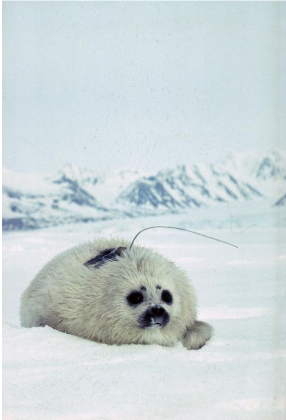
Figure 1 Data loggers can be very small (because power requirements are low), such as this time-depth-recorder (TDR) glued to the fur of this young ringed seal. But, the down side is that such instruments usually need to be recovered to download data. Hence, this pup is also wearing a VHF radio transmitter (with an antenna) to facilitate recovery of the TDR (Photo by Kit M. Kovacs/Christian Lydersen, NPI).
