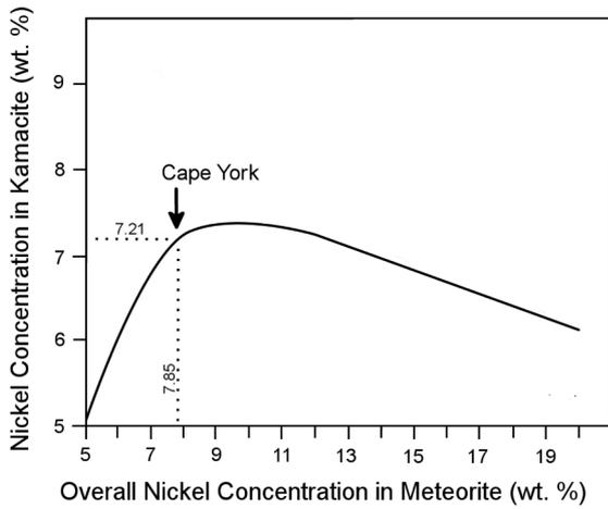
Fig. 5. The experimental relationship between bulk nickel-content of iron meteorites and mean nickel-content of kamacite. Modified after Goldstein (1965). Used with permission of John Wiley & Sons.
