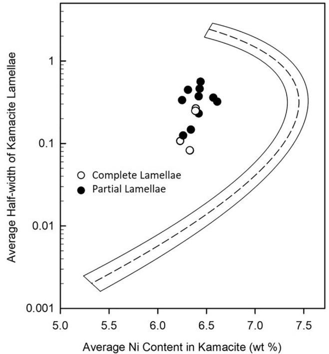
Fig. 8. Data from Table 4 plotted in relation to Goldstein's (1965) curve relating kamacite composition to half-width of lamellae.
