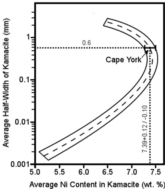
Fig. 6. The experimental relationship between kamacite bandwidth and nickel-content of kamacite. Data from literature values for Cape York are plotted. Modified after Goldstein (1965). Used with permission of John Wiley & Sons.
