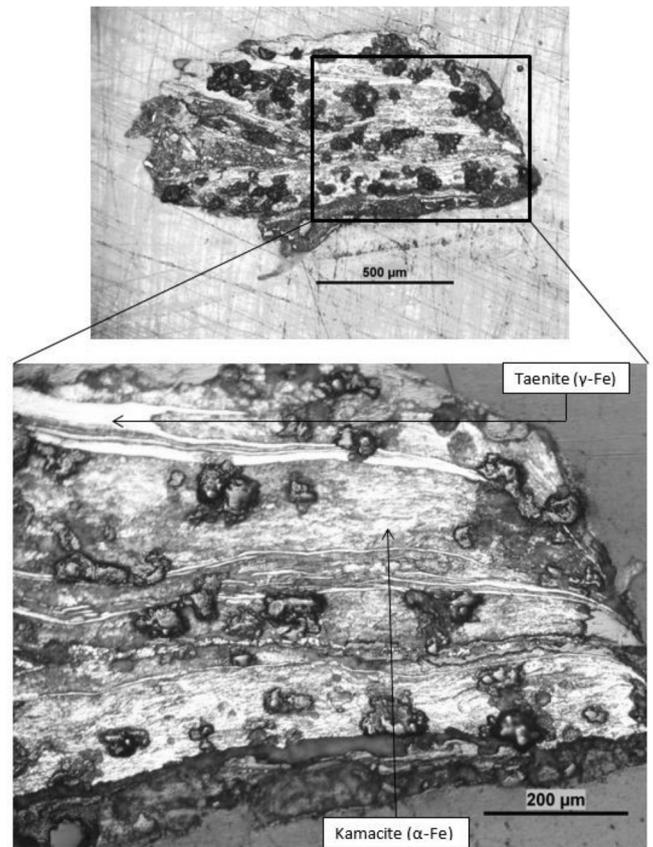
Fig. 4. Polished surface of sample PaJs-2:445 in reflected light with inset showing region analyzed. Note the abundant inclusions of oxidized metal (dark).
