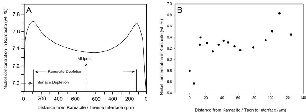
Fig. 3. (A) The M-shaped profile of nickel-content for a typical kamacite lamella. After Goldstein (1965). Used with permission of John Wiley & Sons. (B) Scan across the kamacite lamella of QjJx-1:60.
