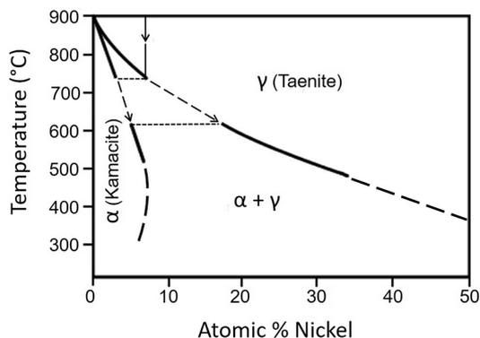
**Fig. 9.** High-temperature phase relations in the iron-nickel phase diagram, after Goldstein and Ogilvie (1965). The arrow shows the cooling path for a typical bulk composition leading to the formation of the Widmanstätten structure, where  $\alpha$  is kamacite and  $\gamma$  is taenite. Used with permission of The Minerals, Metals & Materials Society.
