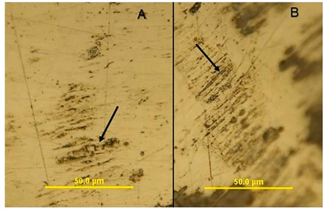
Fig. 7. A) Rhabdite in troilite nodule in reflected light (QjJx-1:71). B) Lamellae of daubr elilite in troilite in reflected light (PaJs-2:280).
