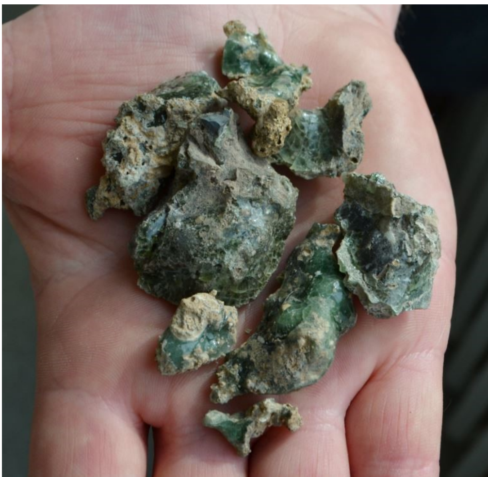
Figure 4: Glassy by product formed inside the furnace of Feature 217.
