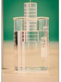
Continue to lower the cylinder in 1 cm increments and record the submerged depths and average forces until the cylinder is completely submerged.
