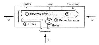
(i) (2 marks) In the forward-active mode illustrated, is the base-emitter junction forward-biased, reverse-biased, or unbiased?
