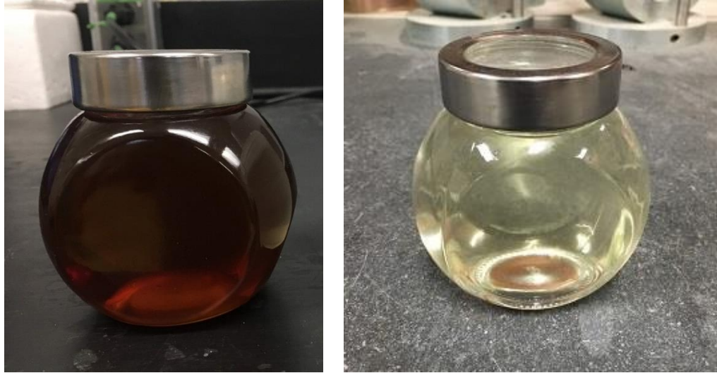
Figure 7 Untreated WCO (left) and Treated WCO (right)
