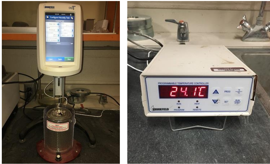
Figure 9 Brookfield Rheometer with Thermosel (left) and Programmable Temperature Controller (right)
