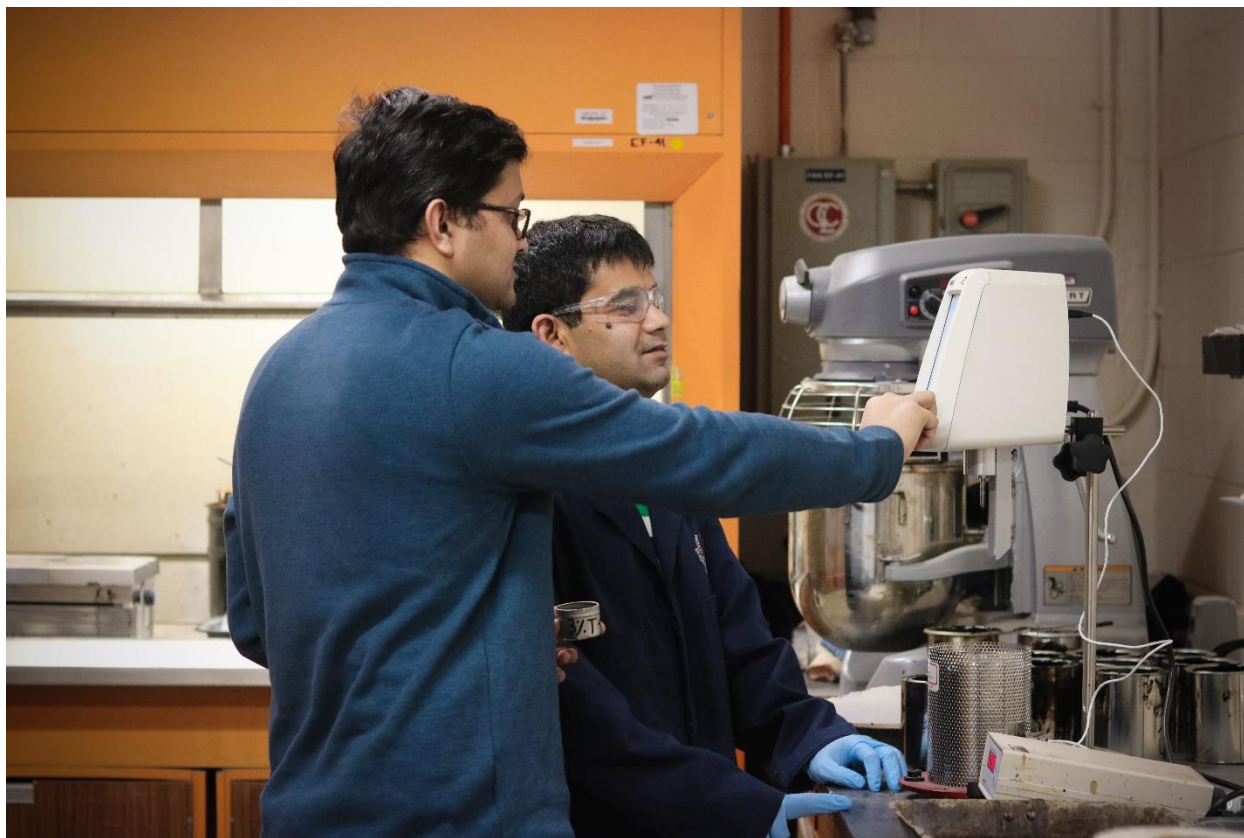
Figure 16 Experimental work on Rotational Viscometer at Asphalt Lab in MUN
