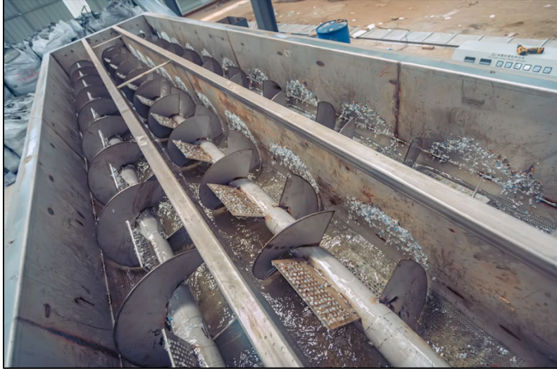
Figure 13: Triple row sink float tank used to wash shredded plastics (ASG, 2020).
