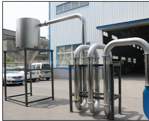
Figure 17: Plastic thermal drying system (MoogTech, 2021).
