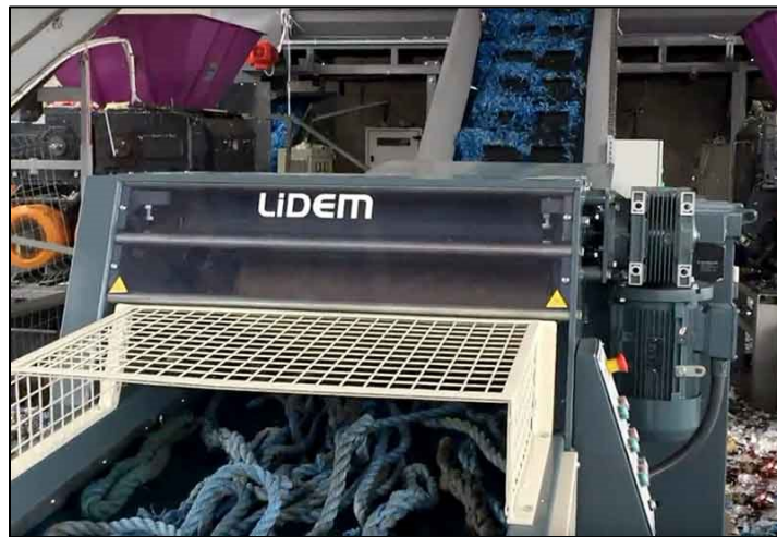
Figure 12: LIDEM rope cutting, chopping, and shredding system. The Rotator (LIDEM, n.d.).
