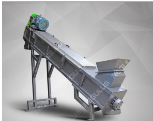
Figure 14: Regulus plastic washing unit. Friction washer (REGULUS, 2021).
