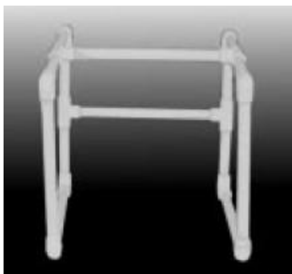
Figure 19 A polyvinyl chloride frame of a processing or preservation chamber (Wilde et al., 2005)
