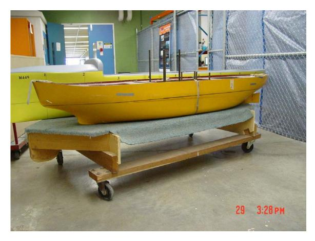
Model Identification:CCGS Sir John Franklin.Model Description:R Class Icebreaker.Research Description:Ice Trials, and Bending moment investigation.
