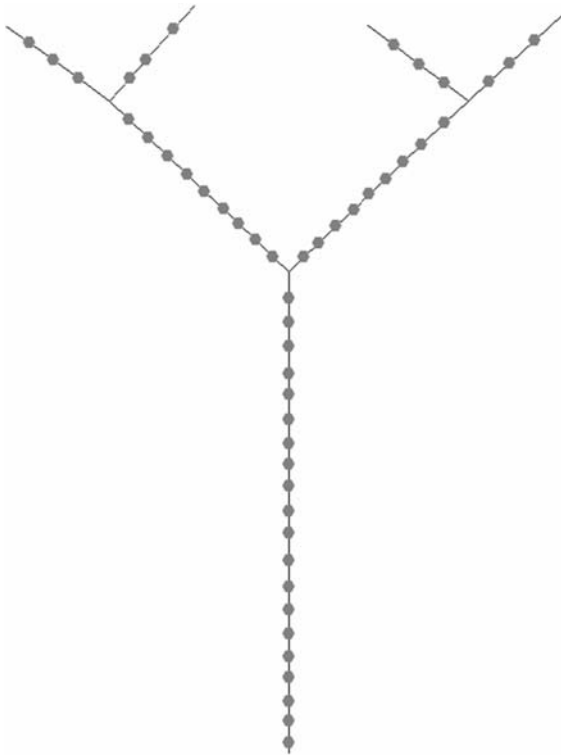
Fig. 2 A simulated three-order dendritic stream network, with 50 systematically placed barriers, used to test the Dendritic Connectivity Index
